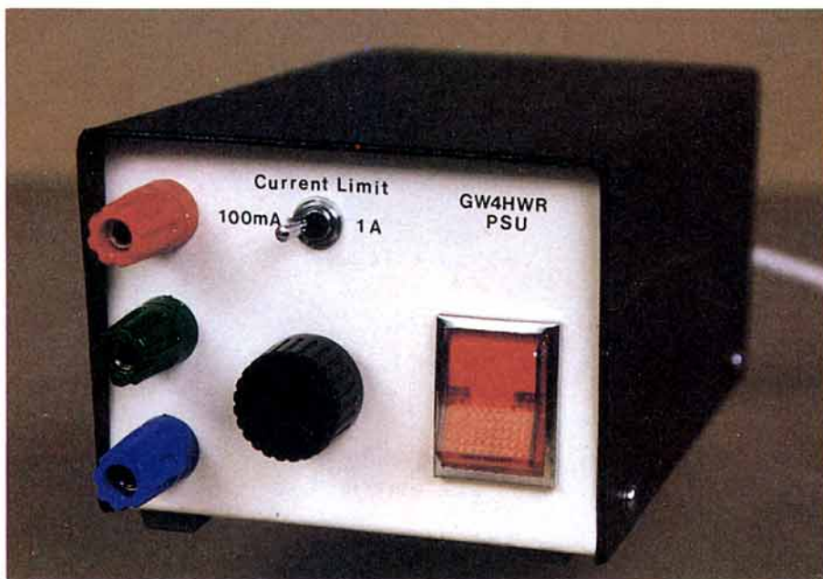
The project itself — a power supply capable of providing one amp at 4.5 to 13 volts.
